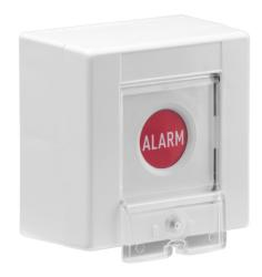
If you press the panic button, you trigger a silent alarm to call for help. You can use the panic button as a standalone device or integrate it into the burglar alarm system. The button is tamper-monitored. For panic and tamper alarms, you have an NO or NC contact. The panic button is VSÖ and VdS C certified.
