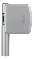
The ABUS FAS101 additional lock is intended for securing the hinge side of a window. You should secure the opening side separately. When you open the window, the FAS101 simply moves with it; in order to tilt the window you must first unlock the security bolt. Then, once the window is in the tilted position, push the bolt back in. The hinge side lock is mounted on the casement and on the frame. Thanks to its narrow design the FAS101 can be used where installation space is tight.
