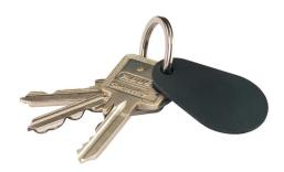
The Proximity Chip Key is an accessory for the Secvest 2WAY and the Terxon SX/MX/LX. Using the Proximity Chip Key replaces entering a code. The Proximity Chip Key is a plastic key with integrated electronic memory. It is programmed directly on the system. To arm or disarm the system, simply hold it in front of the alarm control panel or in front of a Terxon SX/MX LCD control unit. You no longer need a PIN code and thus you can operate your system more conveniently.
