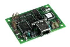
The Ethernet module is an optional add-on module for the Secvest 2WAY. Integrated in the alarm panel, you can use it to send IP-based alarm messages and communicate with the Secvest via the downloader. The Ethernet module is a small, powerful board. It can be quickly and easily plugged into the Secvest.
