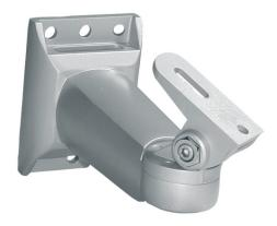
The mount TV8339 is an accessory for the cameras and the IR illuminators from ABUS Security-Center. You can use the mount to attach cameras or IR illuminators to a wall or ceiling. The horizontal and vertical position can be modified with a 1/4" tripod screw. The mount's robust construction prevents that the component attached is simply turned out of position. The mount is suitable for indoor use and outdoor use in roofed areas. Its maximum load is 6 kg.
