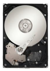
1 TB memory, 140 MB/s data transfer, optimized for 24/7 operations: The new SATA hard disks are the perfect storage medium for your digital recorder.
