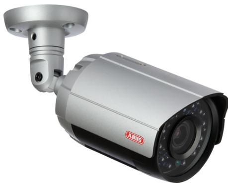
The IR HD-SDI 1080p outdoor camera provides images in full HD resolution, transmitting them as seamless, real-time pictures (uncompressed) via a video cable (co-axial cable). It feeds HD images in 2-megapixel quality to a CCTV system, which are then processed and saved by an HD-SDI recorder. Using an HDMI converter, live images can also be displayed directly on an HDMI monitor or on TV sets.
