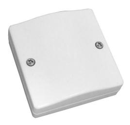
With a screw terminal distributor flush mount, you provide wiring that is clear and easy to understand. Particularly if you install several control panels and sensors, you should fit distributors at the intersections of your building. The surface-mounted screw distributor is tamper-protected by a cover contact. It is produced in white and brown, with 5 (VT5001) and 12 (VT5101) double screw connections. The respective screw terminal distributor flush mount is made of shock-resistant plastic.
