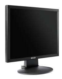
The 17" LED monitor offers outstanding picture quality and fast reaction times for optimum picture fidelity. The integrated BNC connections and other interfaces equip the monitor with requirements for professional video surveillance. The signal is detected automatically, all settings can easily be made in the on-screen display in several languages. Thanks to energy-saving LED technology, the monitor has a low power consumption - and can be used efficiently for 24/7 operation.
