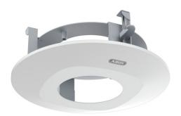
The ceiling mount frame is an optional accessory for IP Dome IPCB72520, IPCB74520, IPCB78520, IPCB72501. When the Universal Dome is mounted in a recess, in the (suspended) ceiling, the mount frame will ensure the camera is stable in position. It also offers an optimum privacy shield, which ensures reliable monitoring both indoors and out. Mounting accessories are provided.
