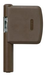
The ABUS FAS101 additional lock is intended for securing the hinge side of a window. You should secure the opening side separately. When you open the window, the FAS101 simply moves with it; in order to tilt the window you must first unlock the security bolt. Then, once the window is in the tilted position, push the bolt back in. The hinge side lock is mounted on the casement and on the frame. Thanks to its narrow design the FAS101 can be used where installation space is tight.
