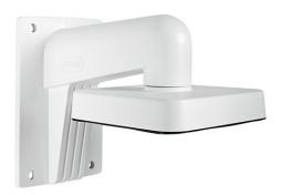
The wall mount is an optional accessory for dome cameras in the "Advanced" series (IPCA). It is used to carry out a professional flush mount of the dome camera in a horizontal position. The sturdy aluminium construction makes it possible for cabling to be both protected and laid internally, and is suitable both for indoor and outdoor use. Compatible with the following models: IPCA72520, IPCA73500 and IPCA76500
