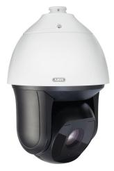
The IP PTZ Dome provides video streams in 4 MPx resolution up to 25 fps. The weatherproof IP66 housing allows outdoor use, due to the integrated IR LEDs the camera can be used at day and night. Access to the camera is always convenient via the Link Station app.
