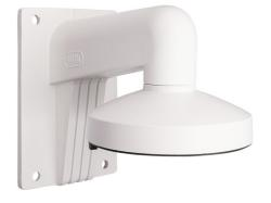
The Wall Mount is an optional accessory for the IP Mini Dome IPCB54511A, IPCB54511B, IPCB58511A, IPCB58511B. It is used to carry out a professional standard flush mount of the Dome Camera in a horizontal position. The robust aluminium design makes it possible for cabling to be both protected and laid internally, and is suitable both for indoor and outdoor use.
