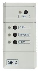
Active glasbreak detectors react more sensitively to glass breakage than passive ones. It is necessary to generate special test signals for each sensor type. Therefore, the glassbreak test instrument is equipped with different functions for active and passive glass breakage detectors. Via a piezoelectric disc on the front of the tester, the test signal is transmitted electromechanically into the pane and sensed by the glassbreak detector.
