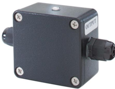
The day/night switchbox is an accessory for the discreet and semi-discreet IR illuminators MEGA LED XL (TV6855, TV6856, TV6898, TV6899). It measures the light intensity in the camera's vicinity and switches on the IR illuminator if light intensity is below 10 lux. Thus, the IR illuminators are only activated if the available light is not sufficient for the camera. This helps to save power and extends the service life of the illuminator.
