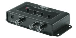
The signal repeater amplifies the video input signal and transmits it without loss over long distances. Install connections via coaxial cables (RG59): From your camera's video input to the signal amplifier and from the signal amplifier's video output to one or two monitors. The maximum distance between the signal amplifier and the monitor is 1000 meters. You can fine-tune the settings such as brightness and focus directly at the signal repeater.
