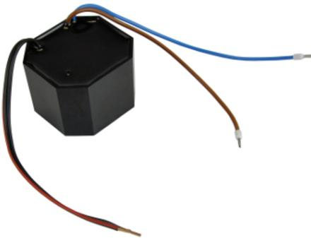
The stabilized mini integrated power supply (230 V AC / 12 V DC, 1 A) supplies power to your video components. With its compact size it is particularly suitable for installation in 55 mm flush-mounted sockets and wherever little space is available for power supply.
