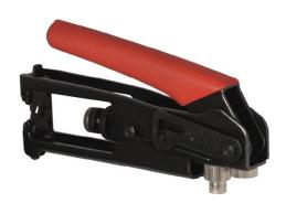
The RG-6 compression pliers are the right tool for working with double-shielded RG-6 coaxial connections. This makes it easy to optimally connect BNC cables to cameras, recorders, monitors, repeaters, or converters. The matching RG-6 coaxial cable is a double-shielded 75-ohm cable that was specially developed for broadband applications (such as HD-SDI).
