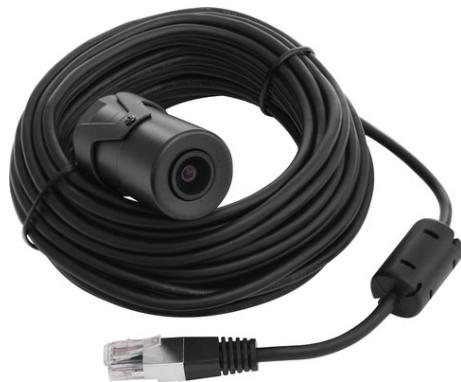
The tube-shaped camera module is a required accessory for the Dual Flex Encoder IPCS10020. The mini module measures just 50 x 26 mm and has an 8 m cable for connection to the encoder, which runs from the back of the device. With an angle of view of 92.5°, the 2.8 mm lens gives a good overview of entire rooms.
