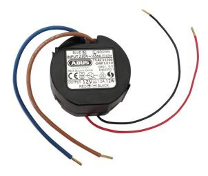
The stabilized mini integrated power supply (230 V AC / 12 V DC, 1 A) supplies power to your video components. With its compact size it is particularly suitable for installation in 55 mm flush-mounted sockets and wherever little space is available for power supply.
