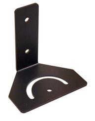
The TVAC31700 Mounting Bracket is an additional, optional accessory for the ABUS TVAC71070 LED Infrared Illuminator. It is used for the professional wall installation of the infrared illuminator for stepless horizontal alignment. The robust stainless steel construction enables secure and stable installation in both indoor and outdoor areas. Note: From summer 2019, ABUS surveillance cameras will also be available with black housing. Please contact us to discuss.
