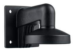
The Wall Mount is an optional accessory for the IP Mini Dome IPCB42510A/B/C, IPCB42515A, IPCB44510A/B/C, IPCB42501, IPCB42551. It is used to carry out a professional standard flush mount of the Dome Camera in a horizontal position. The robust aluminium design makes it possible for cabling to be both protected and laid internally, and is suitable both for indoor and outdoor use.
