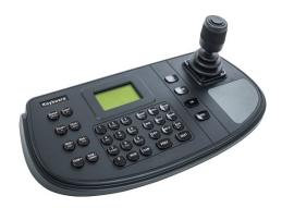
Help yourself! Controllable video surveillance for analogue cameras. This ergonomically designed and robustly made control panel enables simple control of up to 255 motor domes via RS-485 or directly via network. The integrated LCD display enables you to monitor each of your control steps. One special feature is the additional option to directly control several recorders. Direct access to the OSD of the connected dome is also possible.
