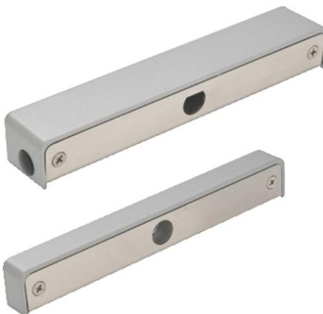
Surface-mounted housing and counterpart for the locking element AZSE10000 and AZSE10100, if it is not possible to mount the locking element in the door frame. The magnet for activating the SpE internal magnetic contact, as well as the additional magnetic contact is included in the counterpart.
