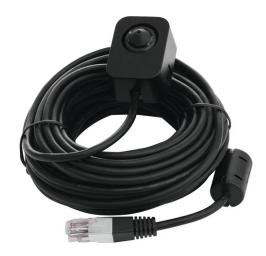
The rectangular camera module is a required accessory for the Dual Flex Encoder IPCS10020. The mini module measures just 27 x 37 x 25 mm (inc. housing and adhesive pad) and has an 8 m cable for connection to the encoder, which is routed downwards. With an angle of view of 57°, the 3.7 mm pinhole lens gives a focused view of selected areas of a room or into corridors.
