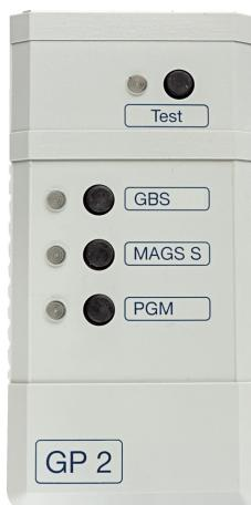
Active glassbreak detectors react more sensitively to glass breakage than passive ones. It is necessary to generate special test signals for each sensor type. Therefore, the glassbreak test instrument is equipped with different functions for active and passive glass breakage detectors. Via a piezoelectric disc on the front of the tester, the test signal is transmitted electromechanically into the pane and sensed by the glassbreak detector.
