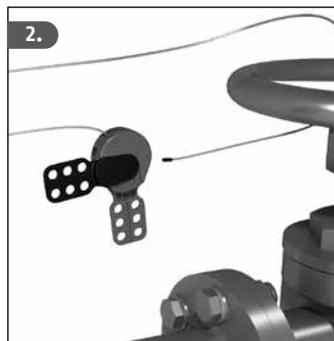
2. Form a loop through the lockout points and insert the cable through the lockout device in preparation for locking the cable into position.
