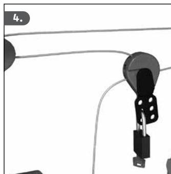
4. Placement of the lock shackle into any one of the six holes will prevent the locking lever from being opened. **Stretch the cable to make sure it is as tight as possible between the locking points.**
