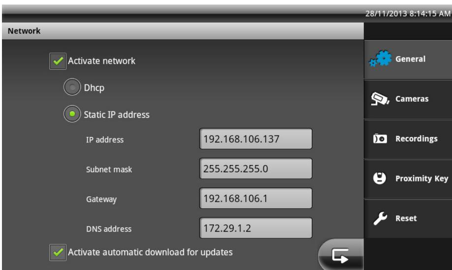
We recommend selecting the DHCP option for internet access (NTP synchronisation). If this causes problems or there is no DHCP server in the network, you can configure a static IP address instead.
