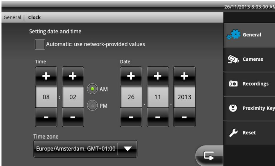
Activate the “Automatic” setting if your Eycasa main unit is connected to your home network (which provides access to the internet). The current time is identified automatically via NTP (Network Time Protocol) any regularly synchronised. Synchronisation takes place once a day or when the Eycasa main unit is restarted.
