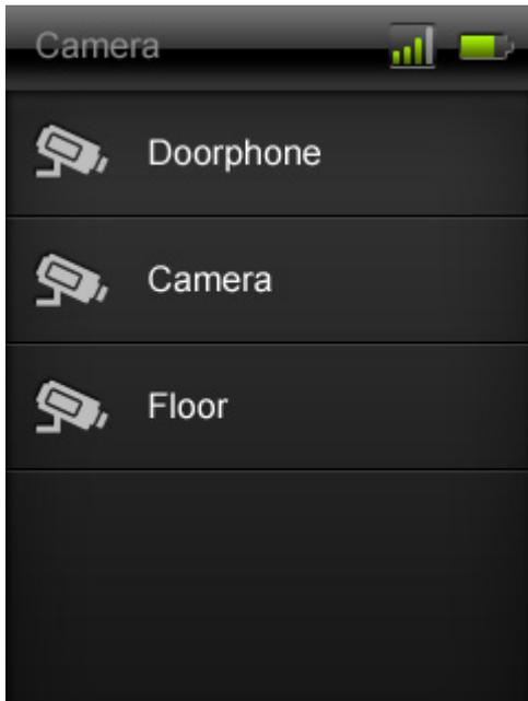
The list visible under “Camera” includes all devices which have been taught in and paired with the Eycasa main unit. The door station and the outdoor camera can be accessed.
