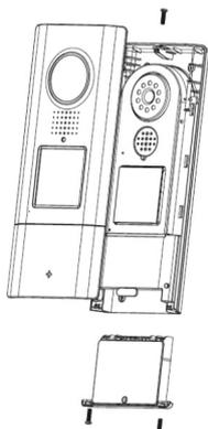
You can now open the plastic cover of the doorbell button and attach your nameplate. For labeling, you can use the included nameplate or the PDF template on the included CD.
