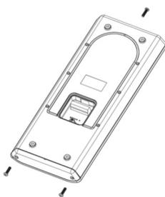
First remove the battery compartment to be able to remove the front cover.
