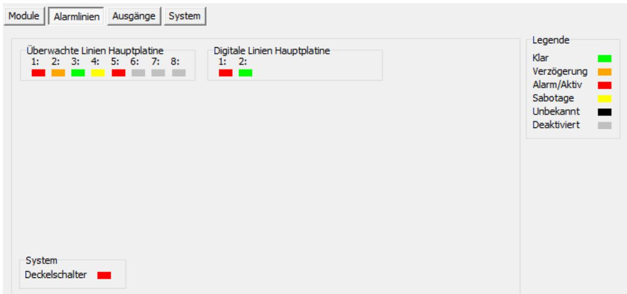
Monitored lines on the motherboard: Eight alarm inputs A1–A8 of the ZWG10200-PSTN/IP CONVERTER motherboard
