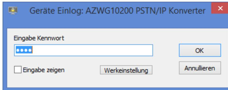
If you do not know the password, the device can be reset using the 'Factory setting' key. **ATTENTION! All programming data will be deleted when this key is pressed!**
