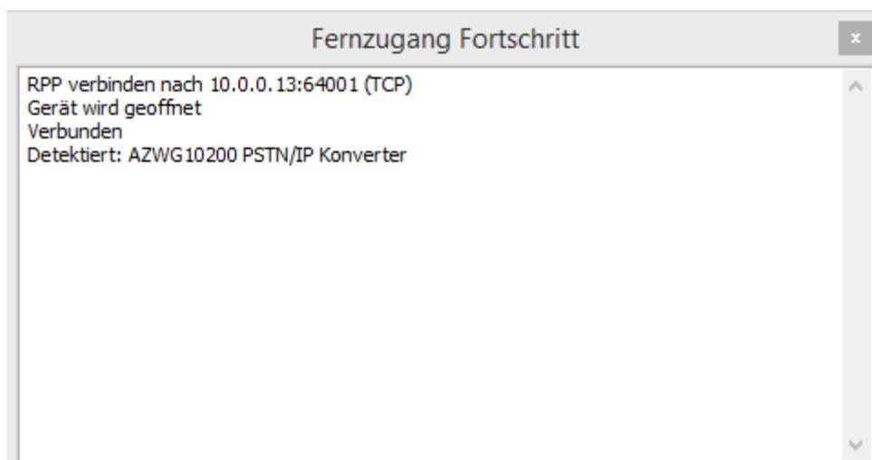
[ParamIt+](#) automatically detects the AZWG10200-PSTN/IP CONVERTER and opens the start screen. The product information is displayed along with the firmware version. The status of the USB or remote connection is indicated at the bottom left of the screen with a green icon.
