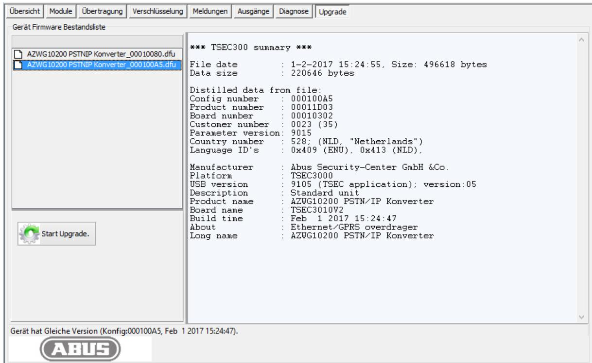
Select the desired upgrade on the left-hand side. Detailed information on the upgrade is displayed on the right-hand side. If the upgrade matches the variant of the AZWG10200-PSTN/IP CONVERTER, the 'Start upgrade' key becomes active. Press 'Start upgrade' and follow the procedure on the screen.
