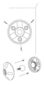
Pre-drill the holes using the drilling template. Unscrew the cover of the wall bracket and mount the floor plate to the wall / ceiling using the supplied mounting material.
