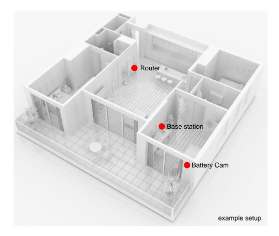
When installing with two cameras, the base station should be centered so that both cameras are within range of the base station. The range of the individual camera to the base station is shown in the live image of the camera by the icon.
