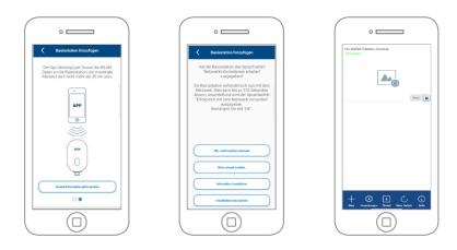
Click on "Send sound information now" to start the transmission. If the transmission was successful, the base station issues the voice command "Receive network information". Confirm this with "OK,
