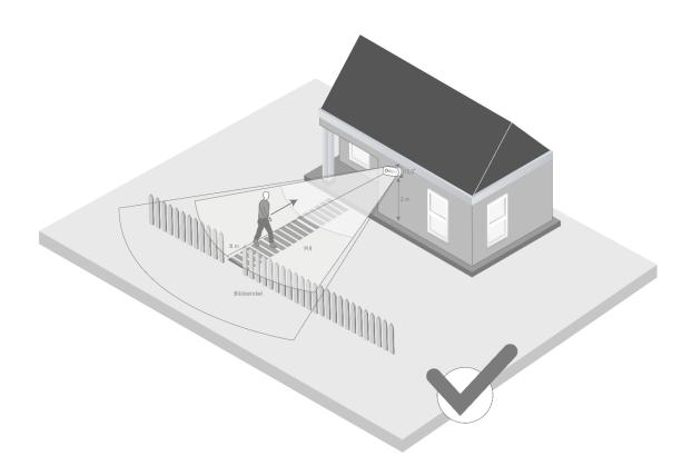
If the movement is detected in the front area of the PIR detection range, the object may not be completely visible on the video sequence.
