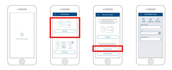
Open the app and click on the "+" to add a base station click on the battery cam. Click on "Existing device" to add the base station already learned in the network to another smartphone.
