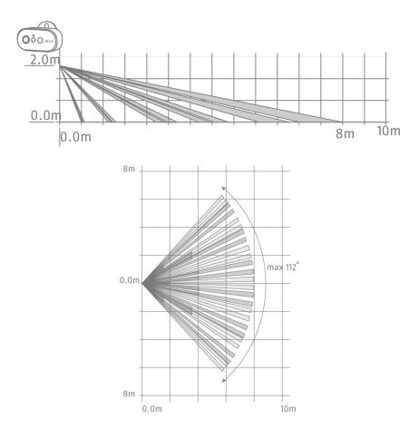
The higher the camera is installed, the greater the downward tilt angle must be. This affects the range of the PIR sensor.
