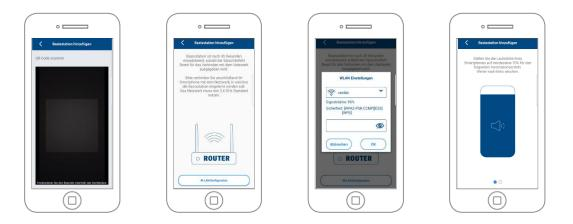
The base station is ready for use after approx. 45 seconds as soon as the voice command "Ready to connect to the network" is issued. Connect your smartphone to the network in which the base station is to be taught-in. The network must use the 2.4 GHz standard.
