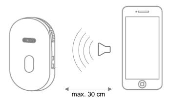
Now set the media volume of your smartphone to at least 70%. In the next step, the app transmits the sound information to the base station. Please note that the distance between the base station and the smartphone must not exceed 30 cm.
