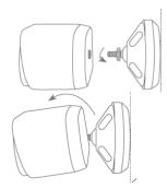
Now screw the fixing ring and the camera onto the bracket. Now you can align the camera using your smartphone. Once the desired viewing angle is reached, screw the cover on tightly.
