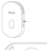
Press the pairing button for at least 3 seconds until the LED flashes blue. The voice command "Ready for Camera Connection" is played. If the camera has already been paired in another base station, please delete it from the camera list in the app beforehand.
