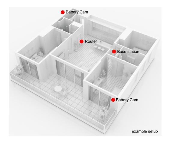
For installations in larger objects with two or more cameras, a second base station (PPIC90010) is recommended to optimize the range.
