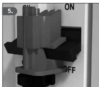
5. If the device sits tightly and securely on the connection bridge of the circuit breaker and prevents the "On" position from being set, turn the screw wheel clockwise until the openings in the screw wheel coincide exactly with the through holes in the lock.
