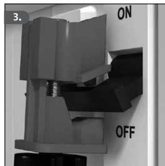
3. Position the circuit breaker lockout device on the circuit breaker so the tongue of the lock engages in one of the spaces between the individual circuit breaker rockers behind the connection bridge.
